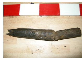
Plate 4 Small wooden fillet hammered in a crack at the end of the mortis joint and tree-nail (411).
